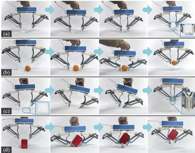
Fig. 12. Experiments of Hoeckens-A Hand: (a) and (b) parallel-pinching of an ID card and an orange; (c) asymmetric scooping of a 0.5mm-thick polyethylene sheet; (d) symmetric scooping and stable enveloping of a 74x110x105-mm tea can.
